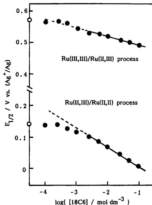
**Figure 3.** Dependence of  $E_{1/2}$  for the redox processes, Ru(III,III)/Ru(II,III) and Ru(II,III)/Ru(II,II), of  $[(\text{NH}_3)_5\text{Ru}(\text{pz})\text{Ru}(\text{NH}_3)_5](\text{PF}_6)_2$  on 18C6 concentration. Open symbols represent the data in the absence of 18C6.
