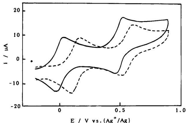
**Figure 2.** Cyclic voltammograms of  $5.0 \times 10^{-4} \text{ mol dm}^{-3} [(\text{NH}_3)_5\text{Ru}(\text{pz})\text{Ru}(\text{NH}_3)_5](\text{PF}_6)_5$  in  $0.1 \text{ mol dm}^{-3}$  TBAH acetonitrile solution in the absence (---) and presence (—) of  $0.1 \text{ mol dm}^{-3}$  18C6.
