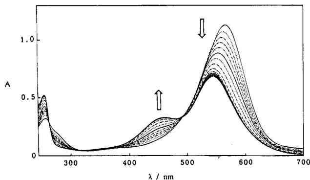
**Figure 1.** Spectral change for the decomposition of  $[(\text{NH}_3)_5\text{Ru}(\text{pz})\text{Ru}(\text{NH}_3)_5](\text{PF}_6)_5$  in acetonitrile at 1 h intervals.  $[\text{complex}] = 5.00 \times 10^{-5} \text{ mol dm}^{-3}$ .
