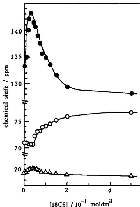
**Figure 6.** Dependence of the chemical shifts of the pyrazine protons (△) and the *cis*- (○) and *trans*-ammine protons (●) of  $[(\text{NH}_3)_5\text{Ru}(\text{pz})\text{Ru}(\text{NH}_3)_5](\text{PF}_6)_5$  on 18C6 concentration.  $[\text{complex}] = 1.0 \times 10^{-2} \text{ mol dm}^{-3}$ .
