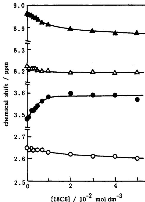
**Figure 4.** Dependence of the chemical shifts of the 2,6- ( $\Delta$ ) and 3,5- ( $\blacktriangle$ ) protons of pyrazine and the *cis*- ( $\circ$ ) and *trans*- ( $\bullet$ ) ammine protons of  $[\text{Ru}(\text{NH}_3)_5(\text{pz})](\text{PF}_6)_2$  on 18C6 concentration.  $[\text{complex}] = 1.0 \times 10^{-2} \text{ mol dm}^{-3}$ .
